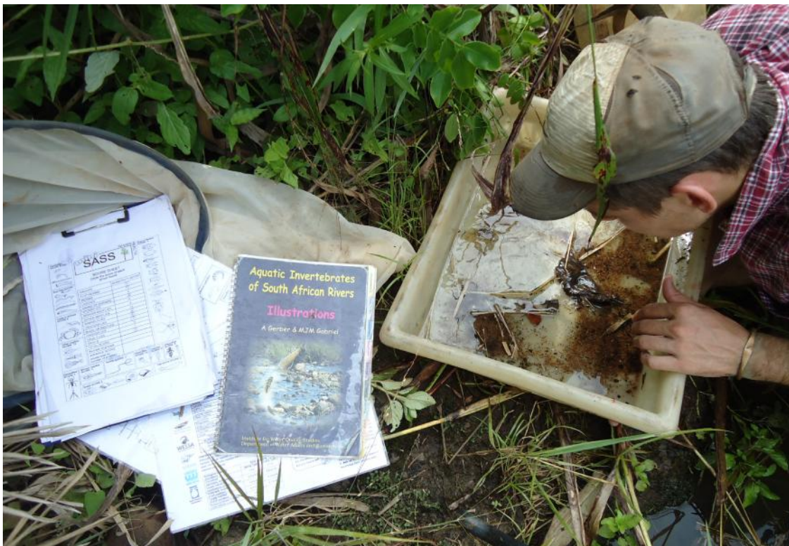
Figure 8: Identification of macro-invertebrates according to the Mini-SASS monitoring protocol.
